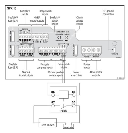
Example of the wiring diagram for the contactor.
