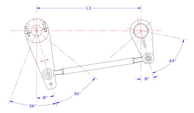
In the table below we show the pedestal to rudder stock distance L3 and the corresponding offset angle B°. If you have instructed us to finish bore and key the tiller arm we will have checked the distance L3 and cut the key-way in the tiller arm to the correct offset angle.
