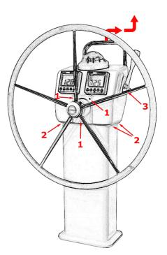
For the ease of mounting the engine control cables (not included), dismount the mechanism by unscrewing it from the bracket (position 1). Do not remove the bracket from the pedestal (position 2) as this bracket is
