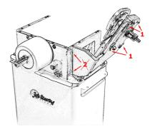
if both the throttle and gearbox levers reach the outer positions and if they are set up correctly in the neutral position. With the red push button one can disengage the gearbox and operate the throttle independently for starting up the engine.
