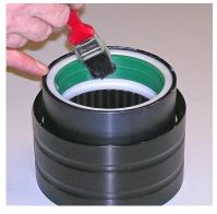
Please note that it is important to visibly check the proper functioning of the lip seals at least once per year, preferably under high pressure conditions like motoring full throttle.
