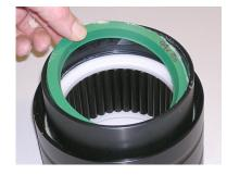
Mount the seal in the housing. This should go quite stiff as the seal should be 0.5 mm bigger than the hole in the bearing. Repeat the same for the second seal.
