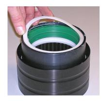
Before you enter the rudder stock, smear some grease on the lips. Don't use too much grease as it shouldn't enter the roller section of the bearing.
