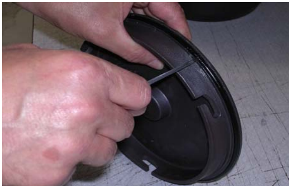
1) Remove the O-ring from the cover.
