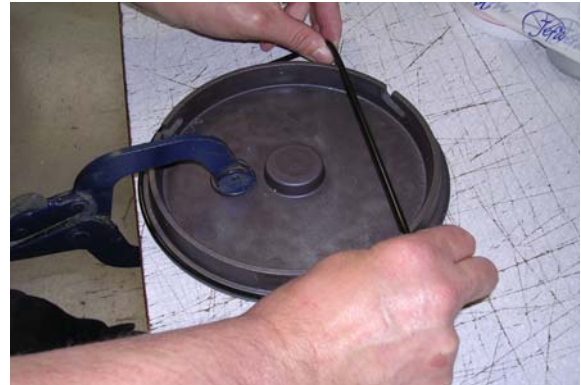
4) Mount the new O-ring on the cover.
