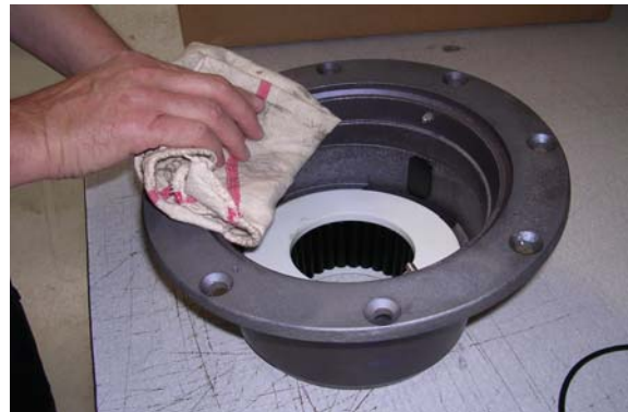
2) Clean the bearing house and cover.
