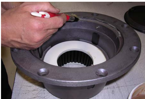
5) Grease the bearing before mounting the cover.
