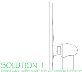
Example 022a: carbon rudder shaft with anodised aluminium or stainless 316 sleeves to achieve an accurate running surface.
