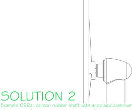
Example 022a: carbon rudder shaft with anodised aluminium or stainless 316 sleeves to achieve an accurate running surface.
