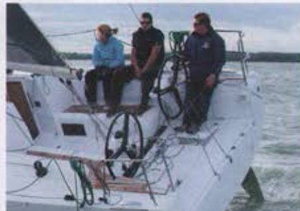
Twin wheels – the popular choice on the Elan 320. A tiller is a money-saving alternative
